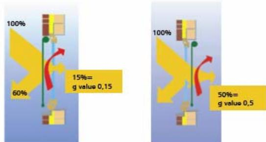
*Exterior vs interior solar shading: typical values*
